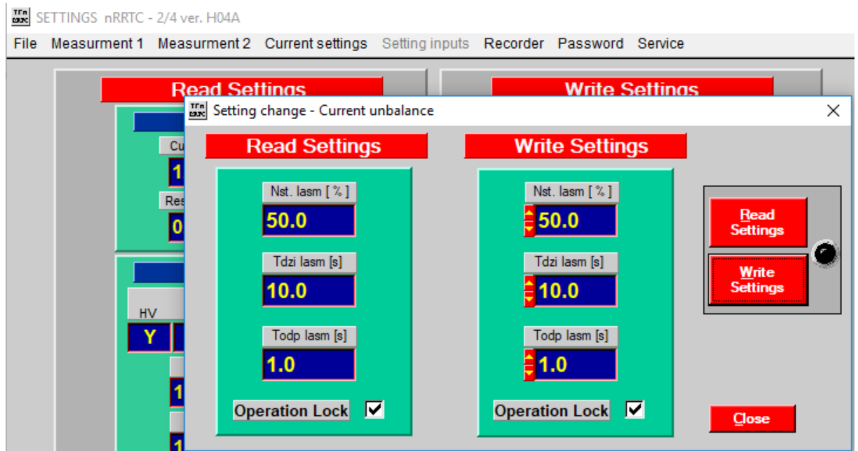
Fig. 7. “Curent asymmetry monitoring” function settings subwindow – function blocked state
